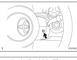
(c) Turn the steering wheel to the right and tighten the screw indicated in the illustration.
